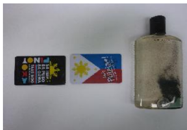
Figure 8. Commercial latch magnets (commonly known as flexible sheet refrigerator magnets), and an improvised magnetic board which is made by filling completely a leak-free, flat container (preferably plastic) with water/mineral oil, and magnetic sand.
