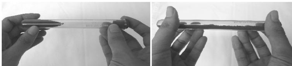
Figure 7a. Leveling the Iron Filings inside the Test Tube
