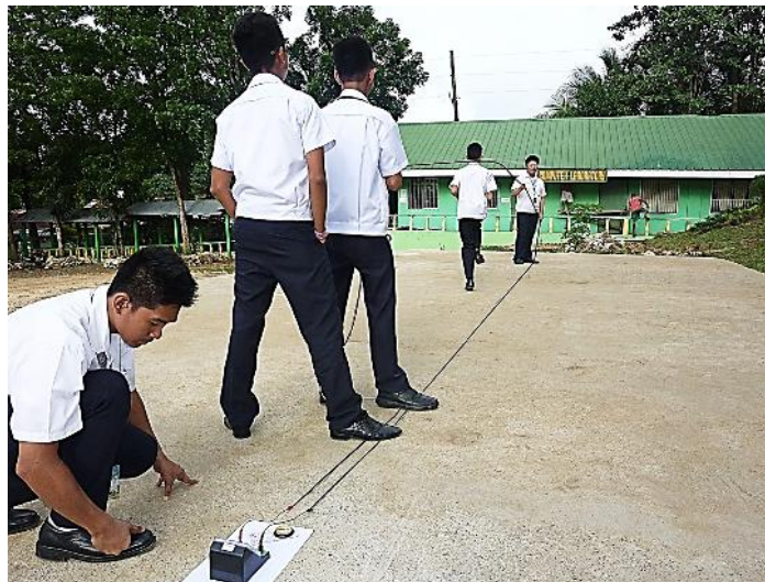
Figure 14. Generation and detection of electricity using the Earth's magnetic field and rotating loop of conductor connected in series to a galvanometer
