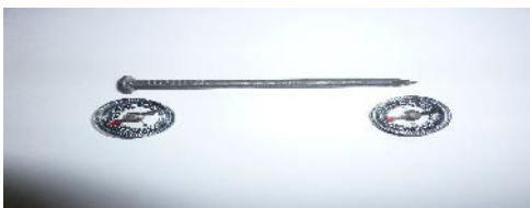
Figure 6. Use of Compass Needles for Checking the Magnetism
