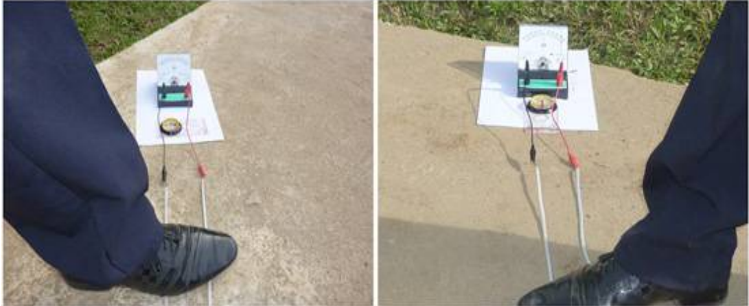
Figure 15. The galvanometer and jump wire electric generator set up along the East-West (left) and along the North-South (right) alignments.
